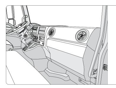
**Step 8:** Complete an install check for the GO device. Once done, reinstall all dash panels.
