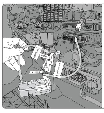
**Step 6:** Plug in the GO device and secure it with the provided zip tie.
