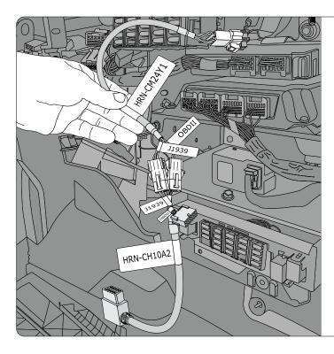
**Step 5:** Plug the HRN-CM24Y1 into the HRN-CH10A2. Be sure to connect both the J1939 and OBD-II 6-pin connections.
