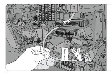
**Step 4:** Plug the HRN-CH10A2 into the factory 10-pin GPS connector.
