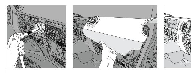
**Step 3:** Remove the upper passenger-side dash panel by removing the two 10 mm bolts.
