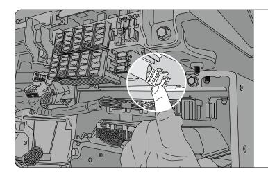
**Step 2:** Locate the 10-pin GPS connector at the back right of the fuse box.
