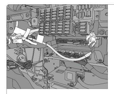
**Step 7:** Neatly run the GO device and cabling to the top dash to the left of the fuse box. Mount the GO device to the factory dash bracket above the fuse box.
