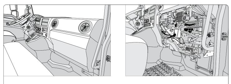
Step 1: Remove the lower passenger-side dash panel. It is held in place by clips only.
